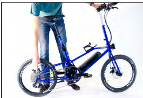
Fig. 2 Shift into middle cog.
