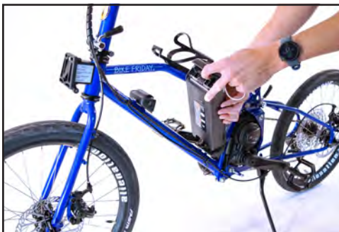
Fig. 1 Insert battery into lower cradle.
