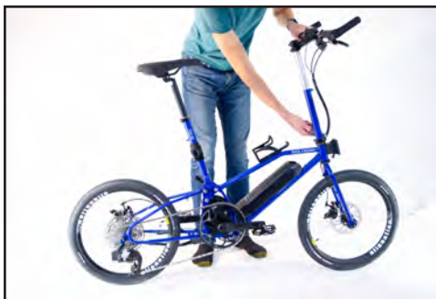
Fig. 4 Loosen stem quick release.
