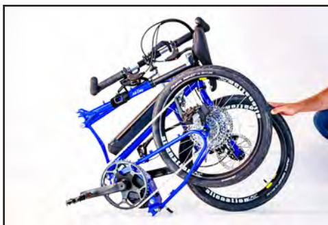
Fig. 9 Nest handlebar on frame.
