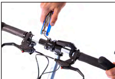
Fig. 19 Tighten handlebar clamp.
