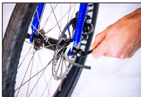
Fig. 2 Setting quick release tightness.
