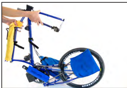
Fig. 11 Turn fork left and fold rear end.
