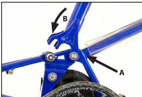
Fig. 8 Engage rear end hinge tips.
