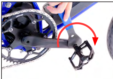
Fig. 27 Tighten pedals (tighten in opposite direction for left pedal).
