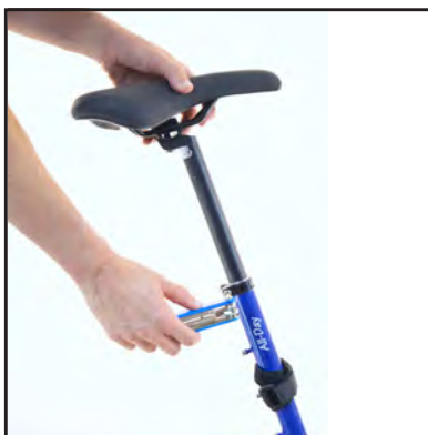
Fig. 3 Remove saddle and seat post.
