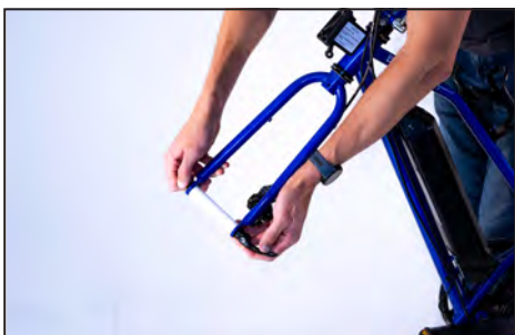
Fig. 10 Remove fork spreader.
