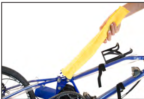
Fig. 10 Fold seat mast forward.
