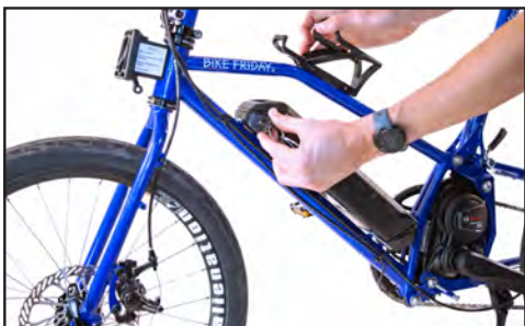
Fig. 3 Unlock battery to remove.
