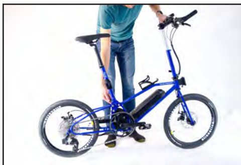
Fig. 5 Loosen frame quick release.
