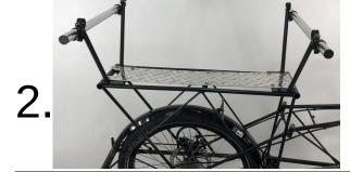
Install (23 inch for HaD, 20 inch for EVD) tubes in front and back of rear rack. The tubes should have 1 inch showing outside of the clamp.
