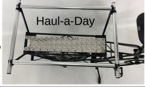
Install 23 inch tubes on either side of the rear rack.
