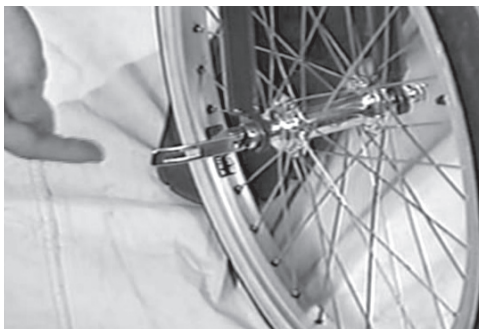
Fig. 1 Quick release operation.
