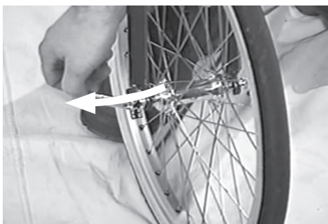
Fig. 2 Setting quick release tightness.
