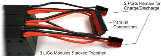
Each battery module has two pairs of +/- leads on them, which are terminated in Anderson Powerpole Connectors. That allows you to string any number of packs together in parallel, with two connectors left open. One connects to the controller and the other could run lights or act as a charging port.
