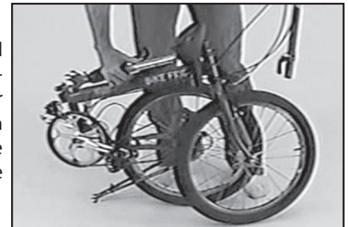
Fig. 9 Fold seat mast past bottle cage.
