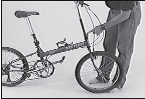
Fig. 4 Loosen stem quick release.
