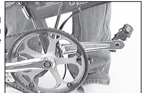
Fig. 3 Left crank arm pointing forward.
