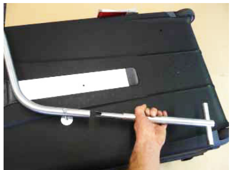
Fig 3. Install trailer tongue.
