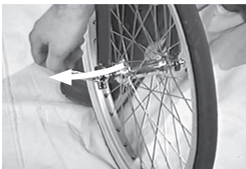
Fig. 10 Setting quick release tightness.
