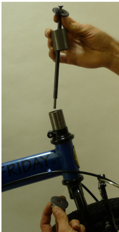
Fig. 46 Headset Press Tool.
