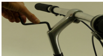
Fig. 30 Quill Stem adjustment.
