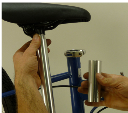
Fig. 26 Lower Seatmast, shim.
