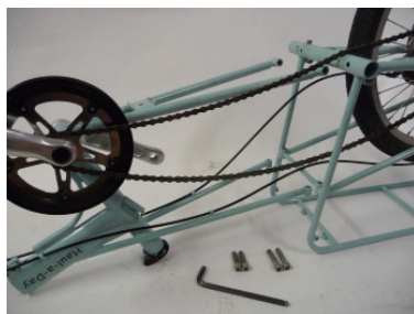
Fig. 3 Place chain on crankset.
