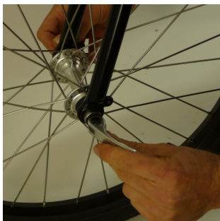
Fig. 12 Front Wheel QR.
