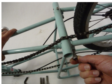
Fig. 4 Hand thread 3/8x16 bolts.
