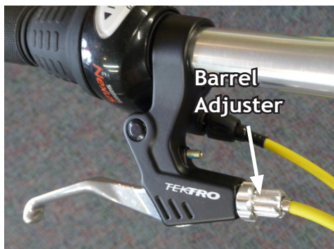
Fig. 20 Brake barrel adjuster.
