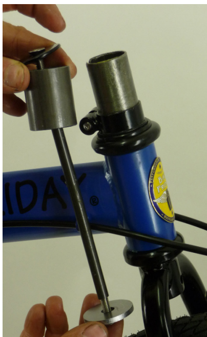
Fig. 45 Headset Press Tool.
