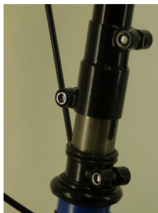
Fig. 24 Mounting stem riser, part 2.
