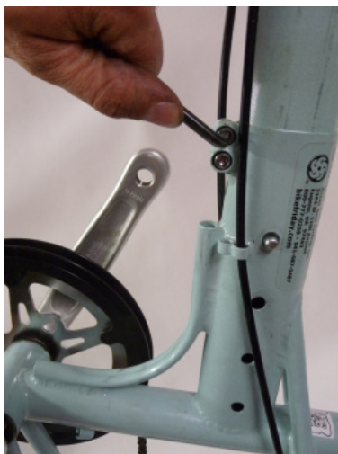
Fig. 37 Loosen pinch bolts.
