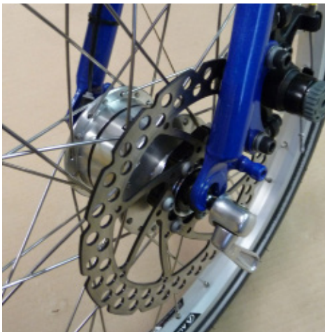
Fig. 17 Insert quick release in wheel.
