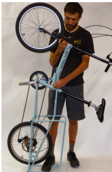
Fig. 38 Loosen pinch bolts.
