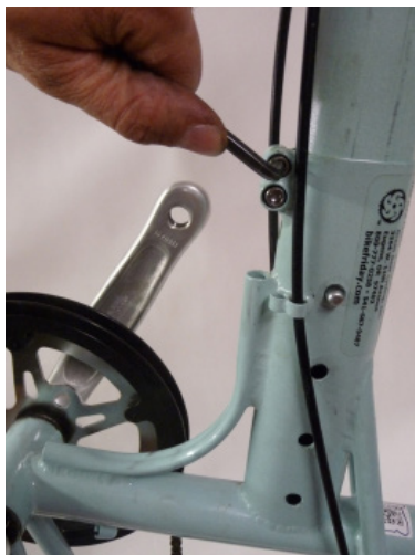
Fig. 7 Tighten pinch bolts.
