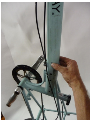
Fig. 6 Insert front section..
