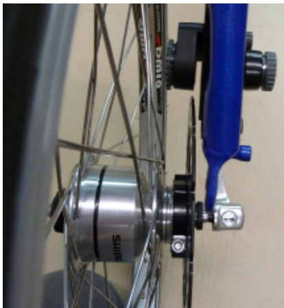
Fig. 18 Disc brake rotor and slot.
