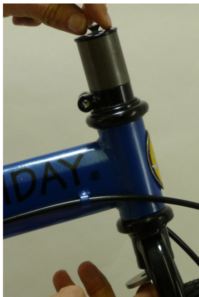
Fig. 47 Headset Press Setup.
