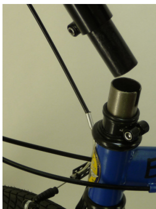
Fig. 23 Mounting stem riser, part 1.
