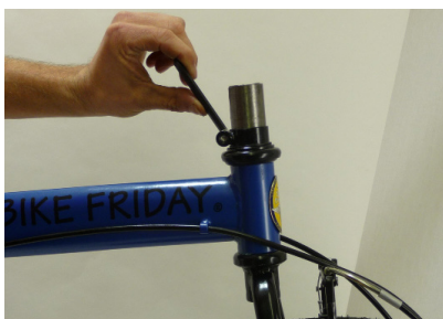
Fig. 42 Loosen Locking Headset Spac.
