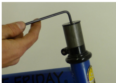
Fig. 48 Headset Press Tighten.
