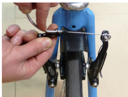
Fig. 15 Slip noodle into slot.
